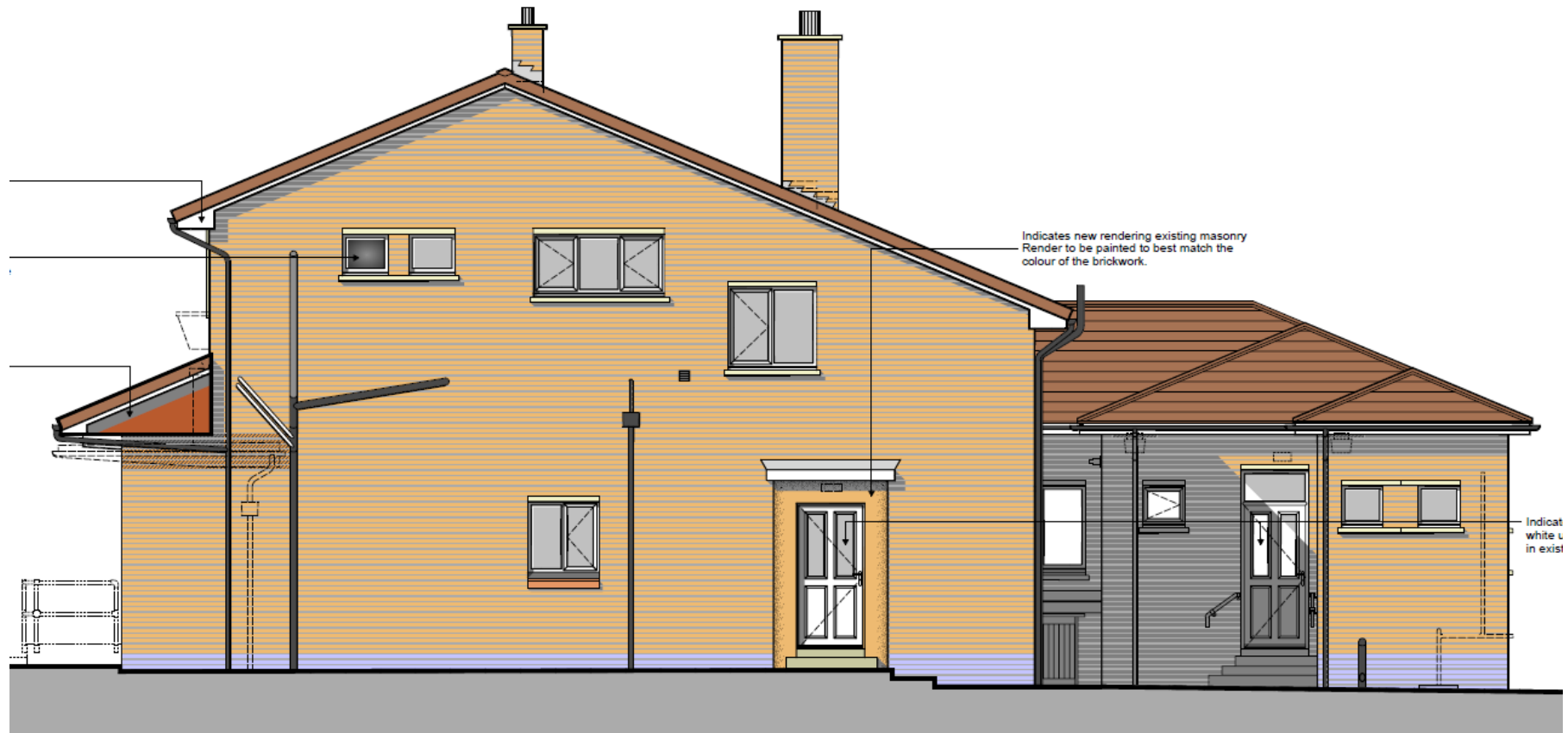
Proposed Side West Elevation (scale 1:50)
